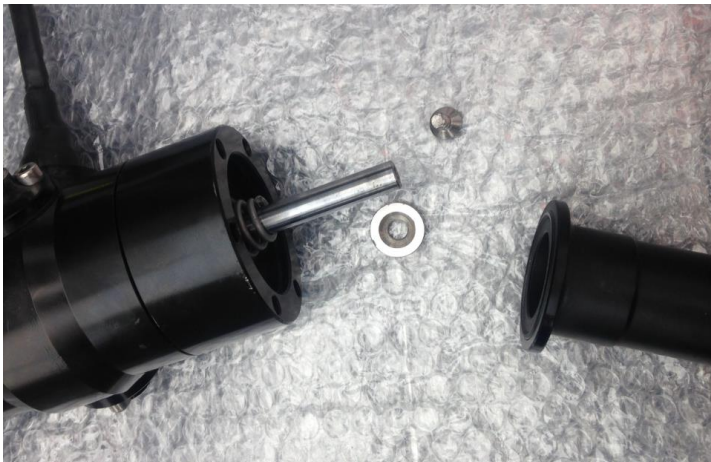
Axle stop screw untighten: no Loctite on.
